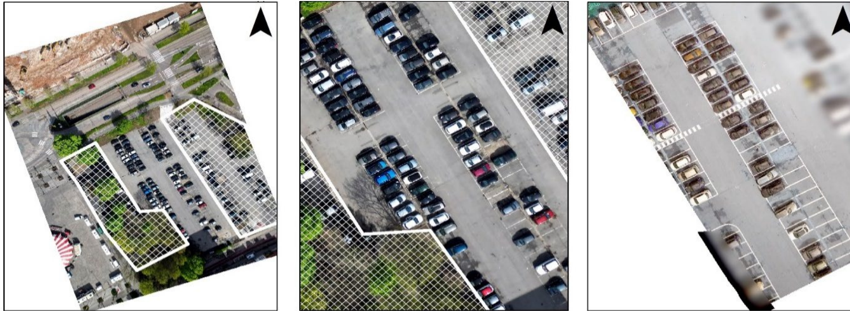
(a) is the template image whereas (b) is the zoomed in area with assumed restricted property for near real-time blurring. Fig.3(c) shows the resulting image from another temporal period (as evident from the lane marking).
